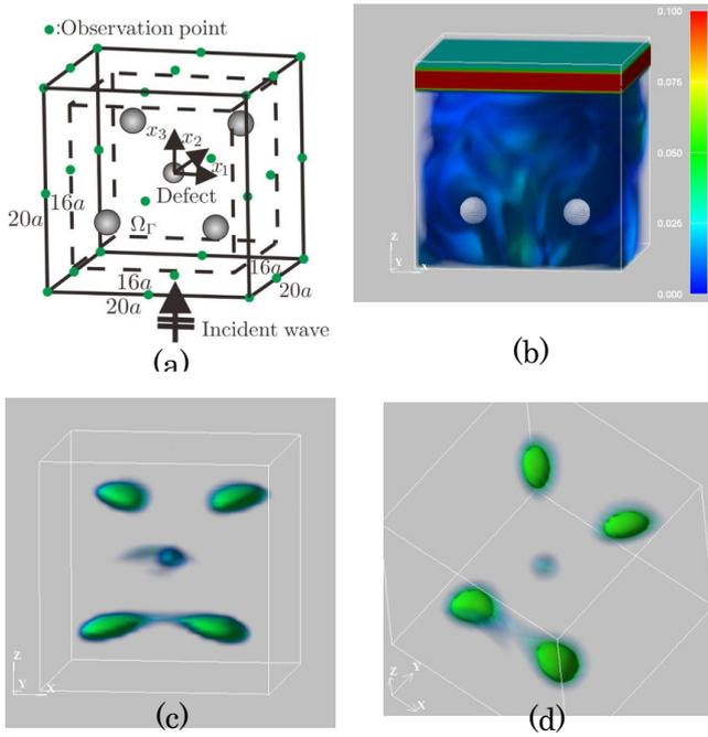
Fig.3: Shape reconstruction of cavities in an elastic solid (a) analysis model (b) a snapshot of elastic wave scattering (c) front view (d) obliquely upward view of the defect shape reconstruction result.
