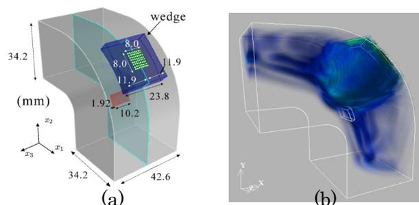
Fig.1: Elastic wave propagation in L-shaped CFRP (a) L-shaped CFRP model (b) a snapshot of elastic wave propagation in L-shaped CFRP.
