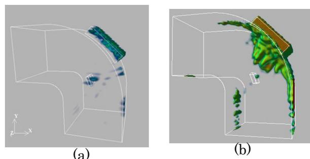
Fig.2: Reconstruction of a delamination in L-shaped CFRP (a) time-reversal result (b) reconstruction result obtained by cross-spectrum.
